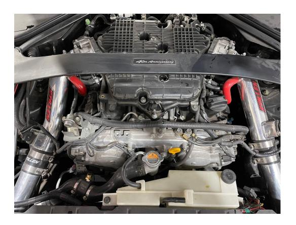
3. Remove the hoses going from the middle of the valve cover to the intake tube or pipe on both the driver and passenger side.
