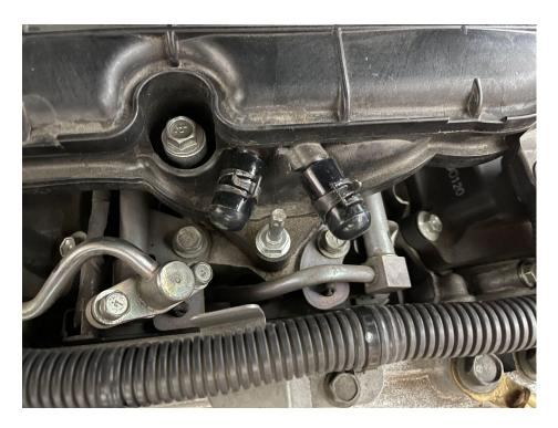
13. Make sure all of your clamps are tight and all of the open ports have been covered by a filter, cap or plug where appropriate. Reinstall your engine cover.
