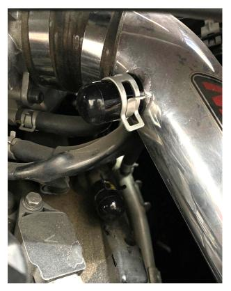
5. Install both of the 1/2in Vibrant filters onto the Vibrant 90 degree fittings and tighten the clamps.
