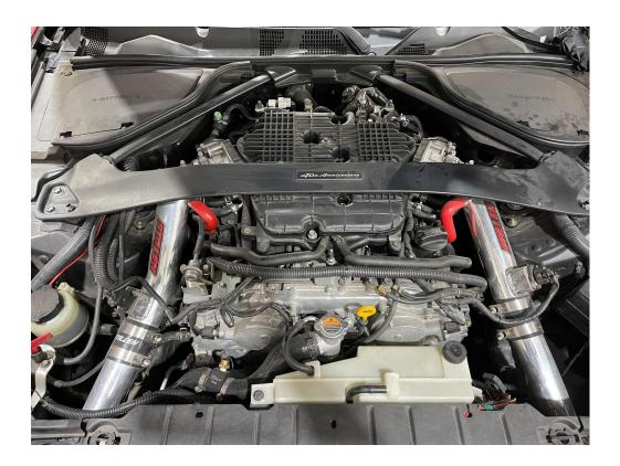
2. Using pliers, slide the clamp retaining the PCV hoses on the front driver and passenger side valve cover off of its barb, do the same for the other side of the hoses on the front of the intake .
