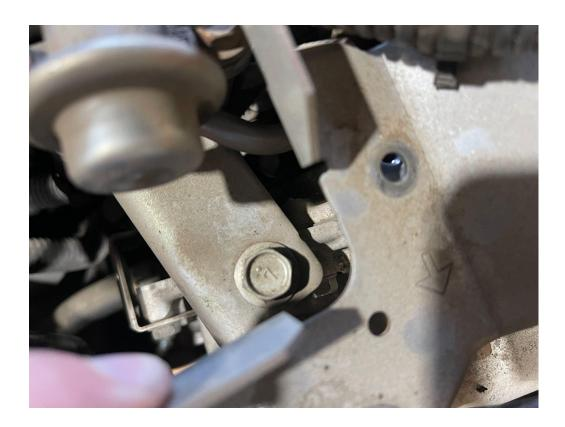
8. Unscrew the stock PCV valves and thread the VQ PCV to -8AN adapters in their place on each of the valve covers and tighten them down snugly. Make sure you oil the o-ring to make sure it goes in and doesn't catch or tear. (it can help to remove the intake coupler for the next few steps but is not strictly necessary)
